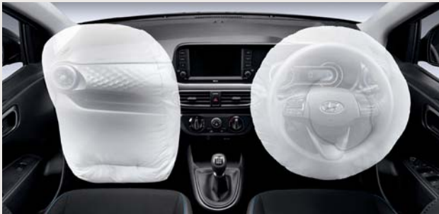
Dual airbag system These newest depowered-type airbags minimize the risk of injuries associated with airbag deployment.
