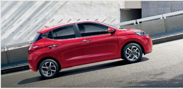
Hillstart assist control HAC maintains braking power after you have removed your foot from the pedal to prevent rollback and releases the brakes the moment your foot touches the accelerator pedal.
